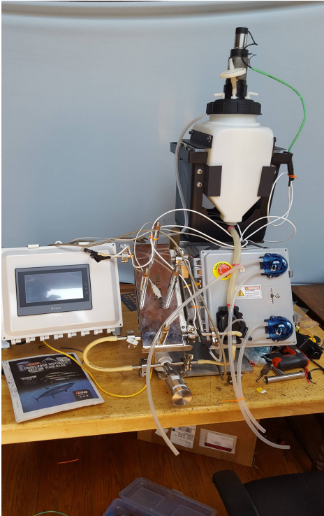
Figure 10. 10L integrated concentration Tank with incline for drainage.
